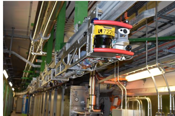
Train Inspection Monorail (CERN made)
