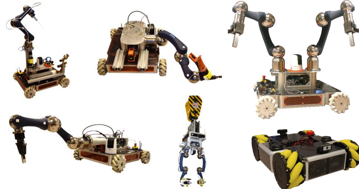
CERNBot in different configurations (CERN made)
