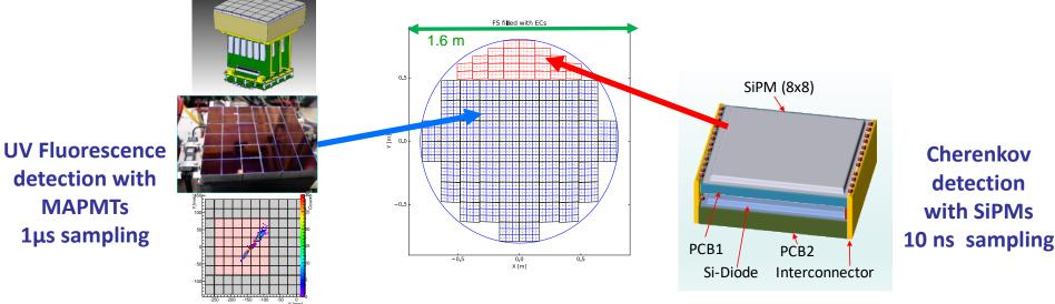
60 Photo Detector Modules (PDMs) = 138,240 pixels 28 SiPM Focal Surface Units (FSUs) =14,336 pixels
