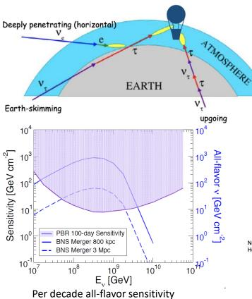
PBR has very limited sensitivity to diffuse neutrino flux, but can observe transients by pointing
