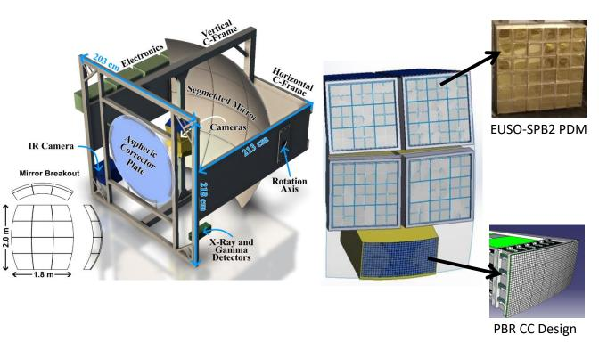
Fluorescence Camera (FC) 4 Photo Detection Modules (R11265 MAPMT): **9216** px
