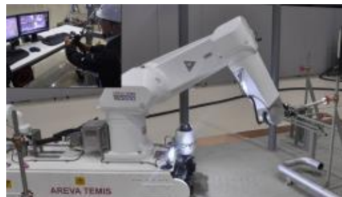
Dexterous operation: Valve opening
