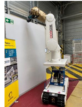
On a mobile crawler and a lifting table (HADE La Hague plant)
