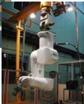
On travelling crane for clean up and waste volume reduction (AD1 facility at La Hague plant)
