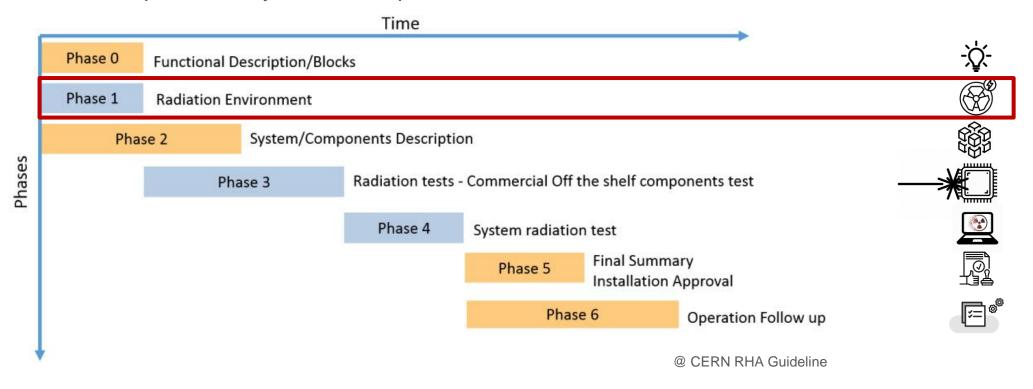
Validation of radiation tolerance at system level before final production
