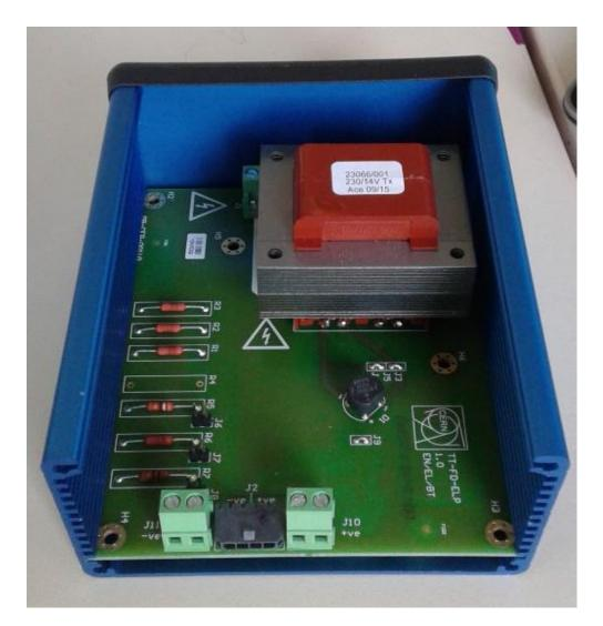
Up to 7W maximum load. Expected functionality up to 1kGy, mixed field. (Limited by Si diodes)
