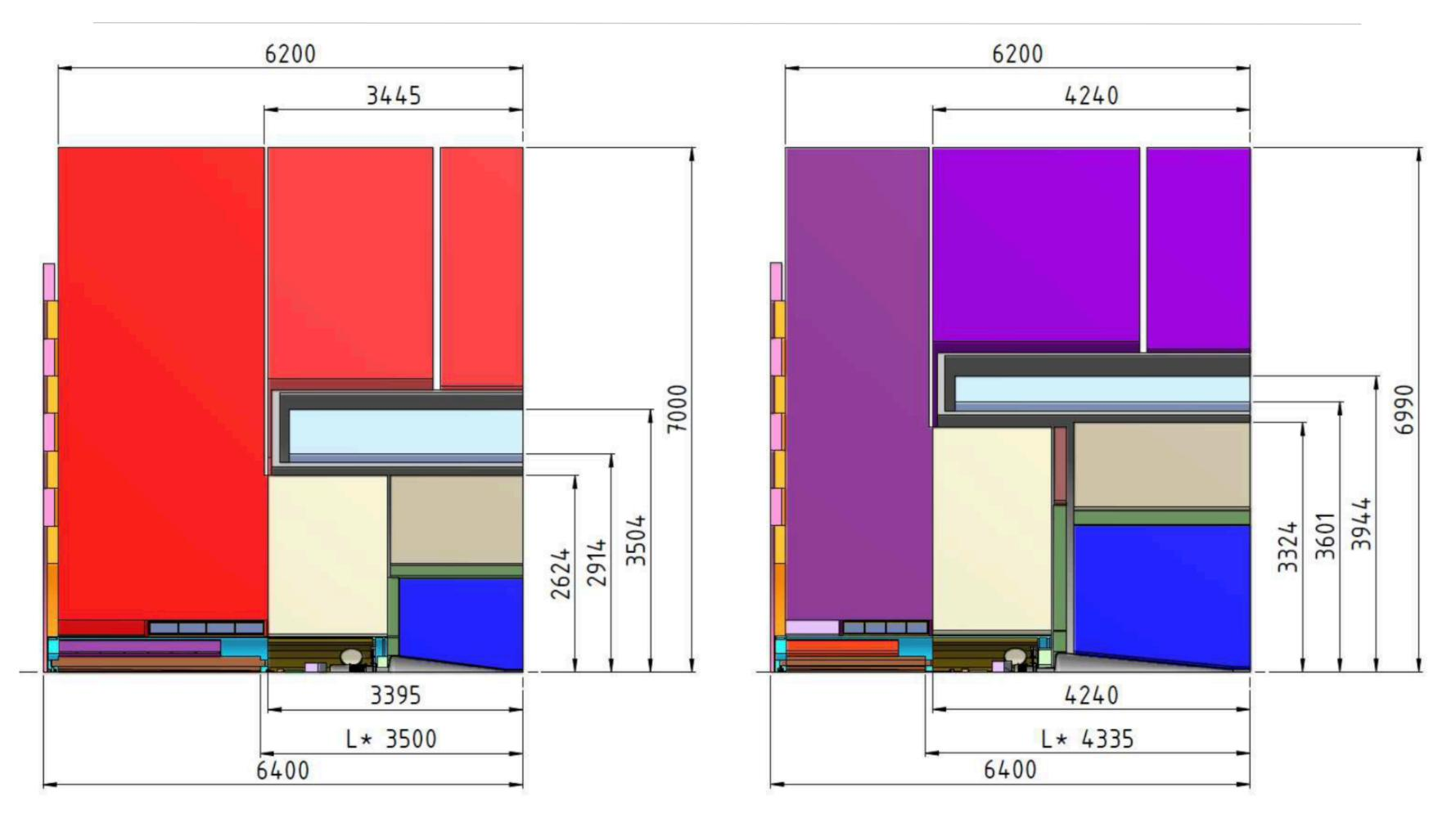
$\neg$  Large and thick solenoids, 5 and 4 T respectively, with anti-solenoids for focusing quadrupoles
