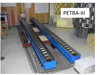
Damping wigglers can be one way of increasing the synchrotron radiation emission.
