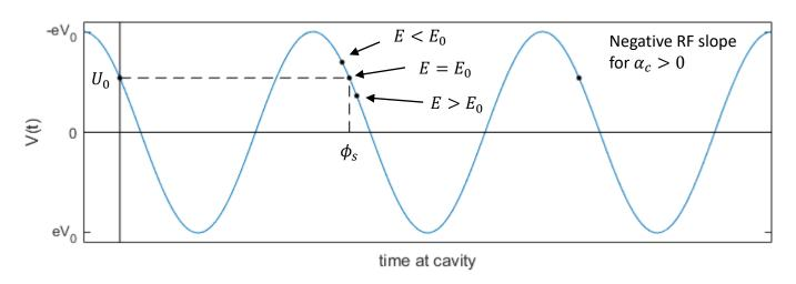
Particles which are high in energy travel further in single revolution and will arrive later Particles which are low in energy travel less distance and will arrive earlier
