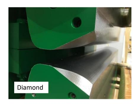
Combined-function bending magnets have both a main dipole field for steering the beam, with a gradient super-imposed on top.
