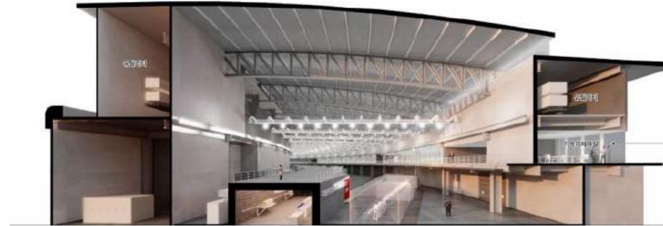
Booster and storage rings share a same tunnel
