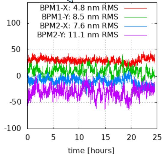
DBPM<sub>3</sub> Drift Test: SLS Hall Ambient Conditions
