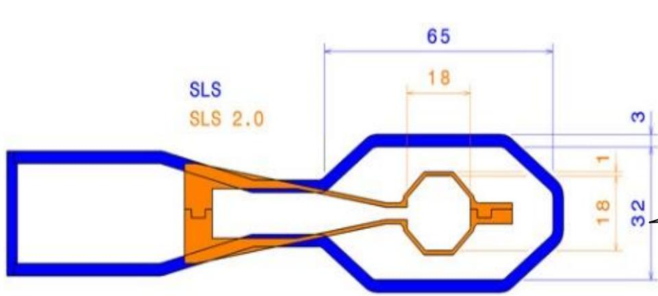
Same BPM electronics has >2x better resolution at SLS 2.0 compared to SLS 1.0
