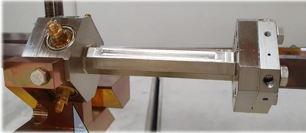
Water cooled copper block reduces position drift
