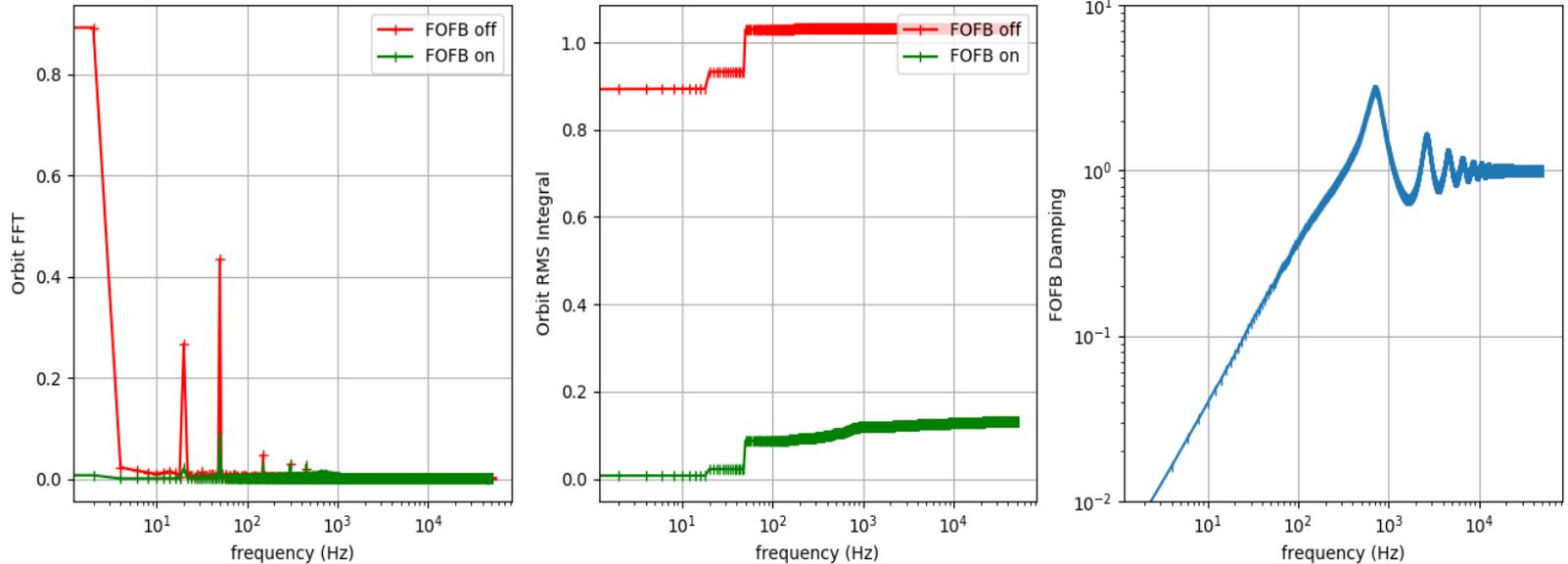
Simulation of SLS 2.0 FOFB correction bandwidth of 324 Hz, assuming 3 kHz BPM and corrector bandwidth, and 0.5ms system latency (= conservative assumptions, may get better).
