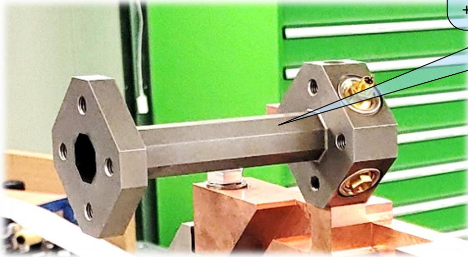
Combined BPM + orbit corrector dipole magnet beam pipe (taper 18→21 mm = synchrotron radiation shielding). 0.5 mm steel + 5  $\mu$ m Cu + 0.5  $\mu$ m NEG)
