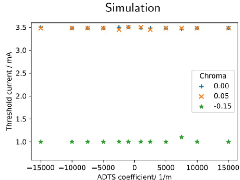
→ No significant influence of ADTS coefficient on threshold current observed
