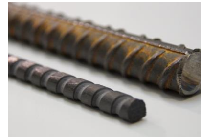
Comparison reinforcing carbon and steel (from https://www.carbocon.de )
