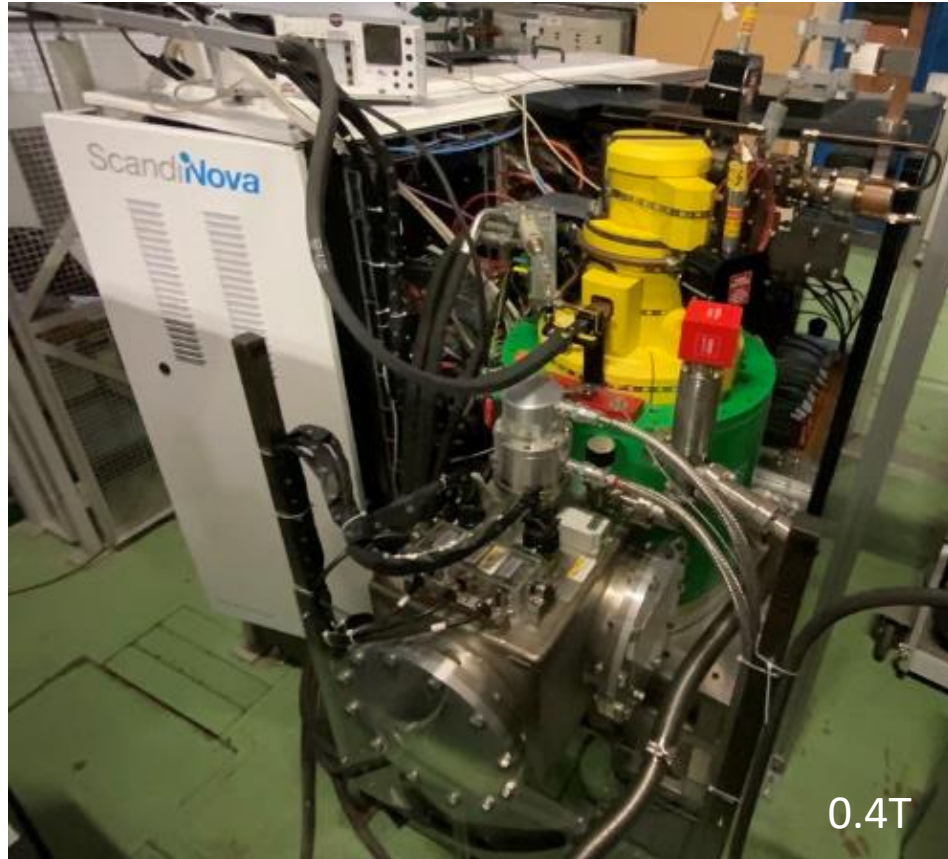
Superconducting MGB2 (28 0 K) solenoid, with the 50 MW X-band klystron, installed on the modulator in XBOX#2. Power consumption reduced from 20kW to 3kW.
