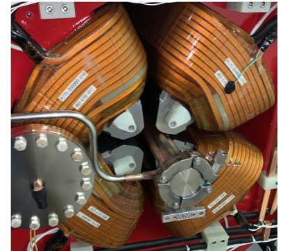
Beam pipe offset 1.28 cm inboard (beam into page)
