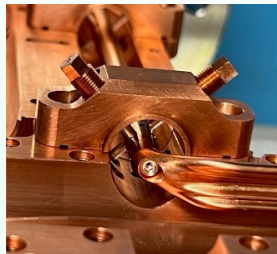
Blade transition and coaxial feeding line suspension
