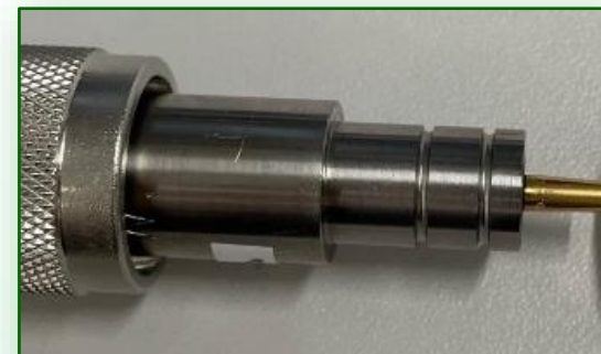
Orient microwave feedthrough.
