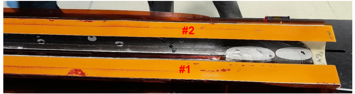
Coil 212: after correction with epoxy resin adhesive (stycast)
