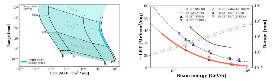
Single species (lead) beam of variable energy and LET, covering the ~10-40 MeVcm<sup>2</sup>/mg range with high energies/penetration Lighter ions are being considered to cover lower LET region
