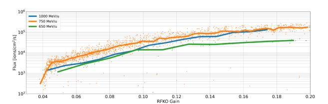
Note: RFKO technique developed and employed for ion slow extraction now also used to improve proton spill quality
