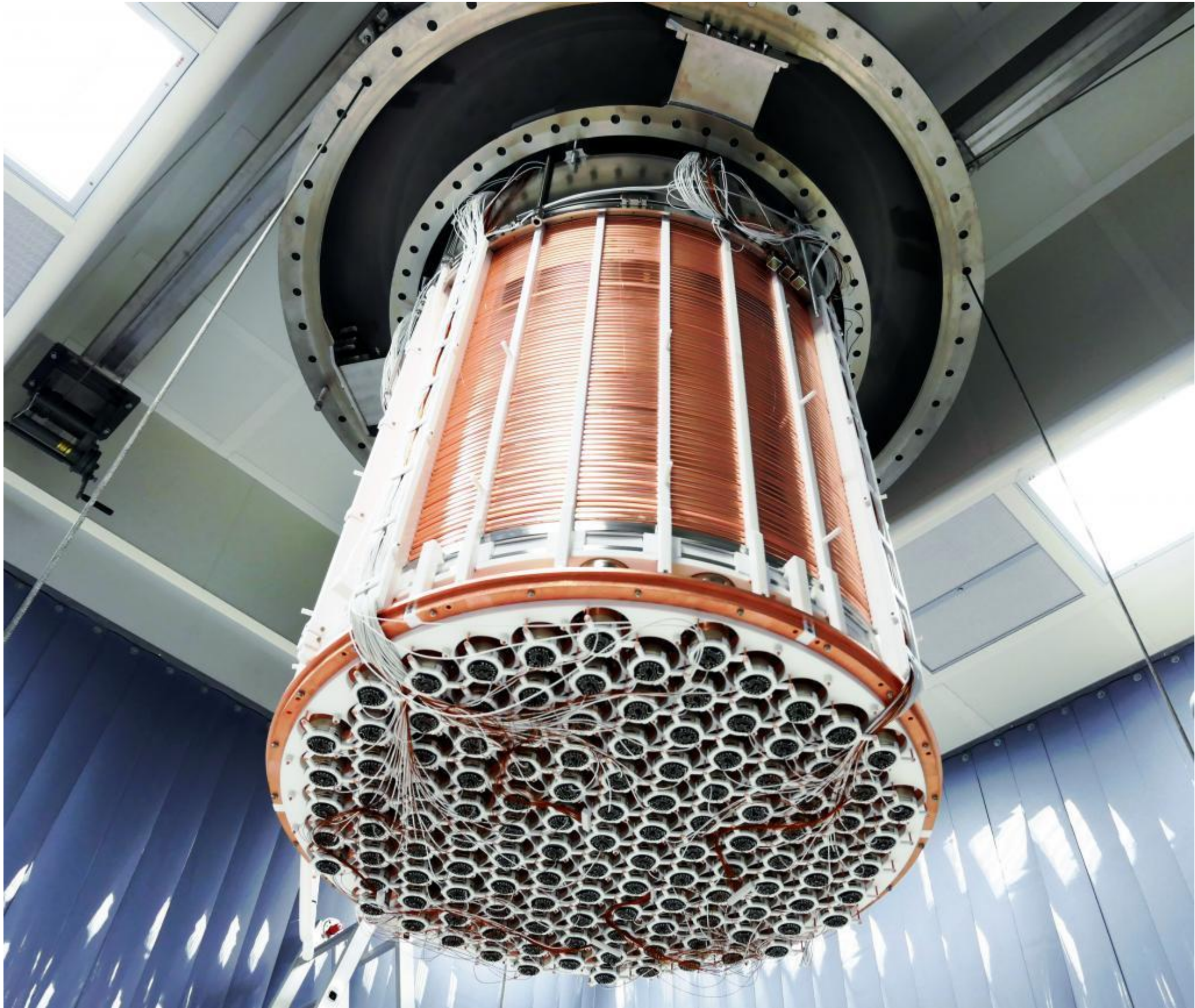
Ultrapure liquid Xenon with light sensors
