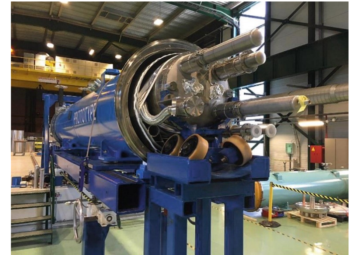
The first 5.5 m long 11 T MBH dipole prototype in its cryostat at CERN ready to be transported to the test bench
