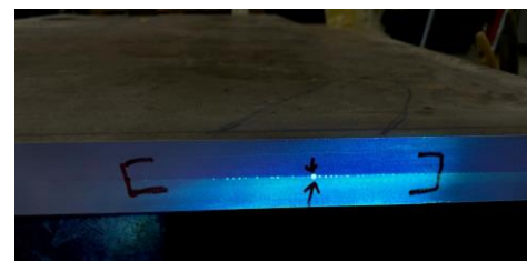
Welds of cryostat in WA105 neutrino experiment
