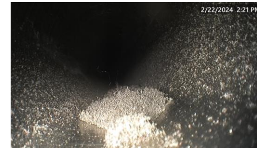
Monitoring the cleanliness of a cooling serpentine in a magnet thermal screen 2 m away of the entry
