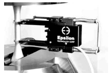
Extensometer under calibration with 12 mm starting length (mass = 0.5 g).
