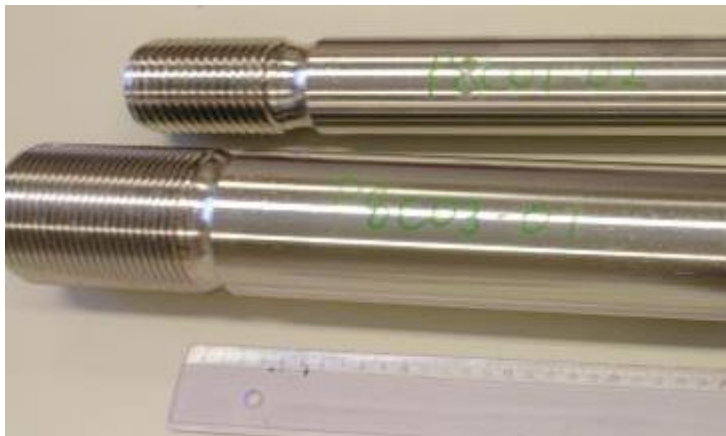
Inconel 718 for ITER magnet supports.
