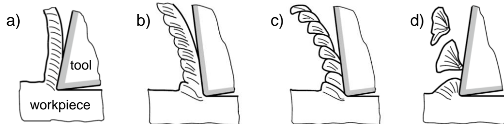
Different types of chip formation; a) continuous chip; b) lamellar chip; c) segmented chip; d) discontinuous chip
