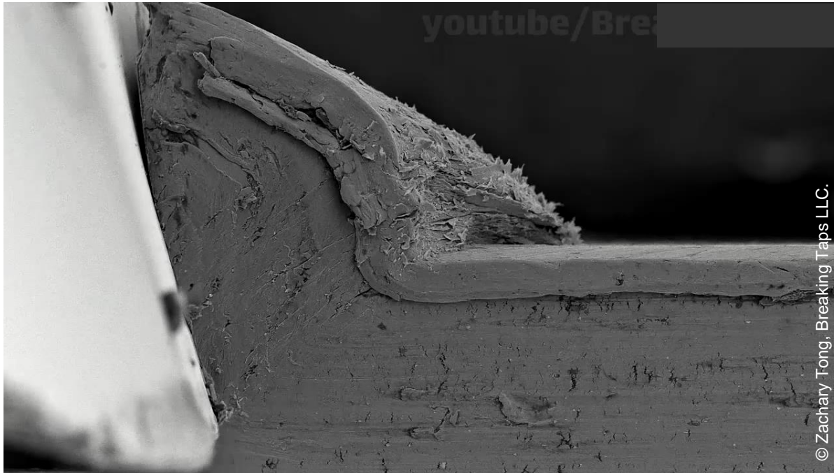
SEM-Images of a ductile cutting process of AlMgSi0.5
