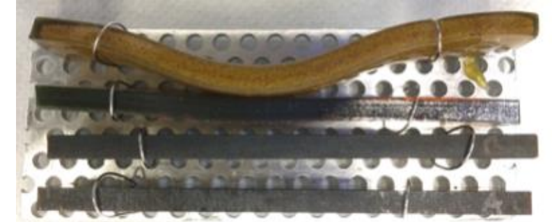
Materials candidate for the protective covers of magnets after gamma irradiation at 10 MGy. Courtesy of C. L. Marraco Borderas [10]
