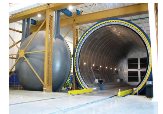
A large autoclave that is used to make the wings of Boeing 787
