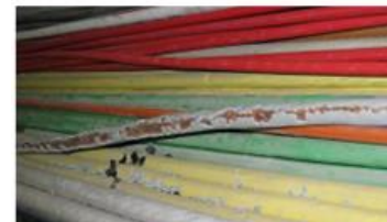
Representative examples of installed cables subjected to different total absorbed dose. CARE Project. Courtesy of J. Gascón [15]
