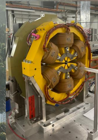
PSI – Sextupole & Octupole Upgrade SLS
