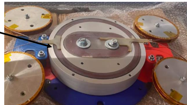
Nb-Ti coils and aluminum pre-compression structure
