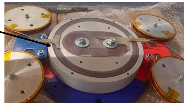
Nb-Ti coils and aluminum pre-compression structure
