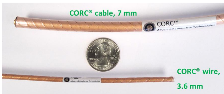
First round, isotropic YBCO wire Courtesy Danko van der Laan (Advanced Conductor Technologies)
