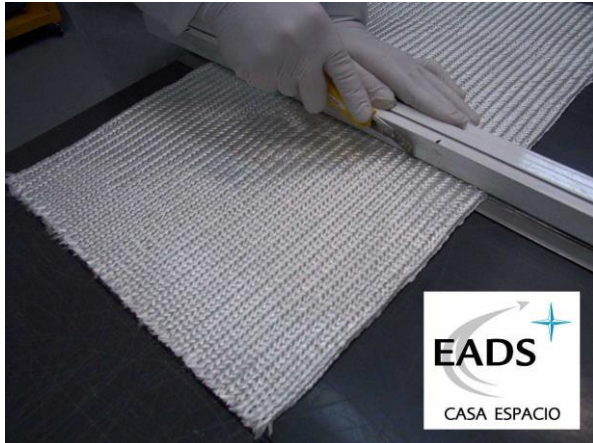
Cutting the fabrics to length
