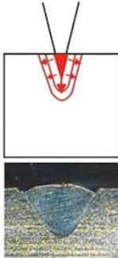
Transition "keyhole" welding
