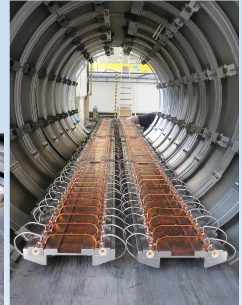
18000 brazing for the thermal links
