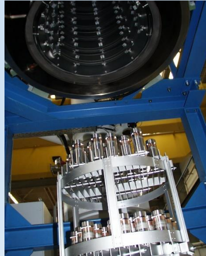
Hundreds of Cu/Stainless steel junctions
