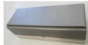
LHC TDI Boron Nitride block
