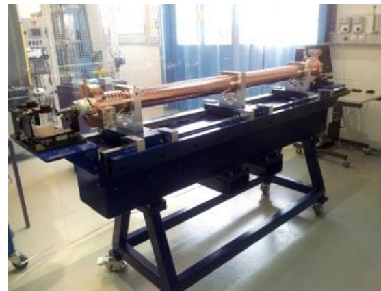
6 GHz TW-SwissFEL After brazing at PSI
