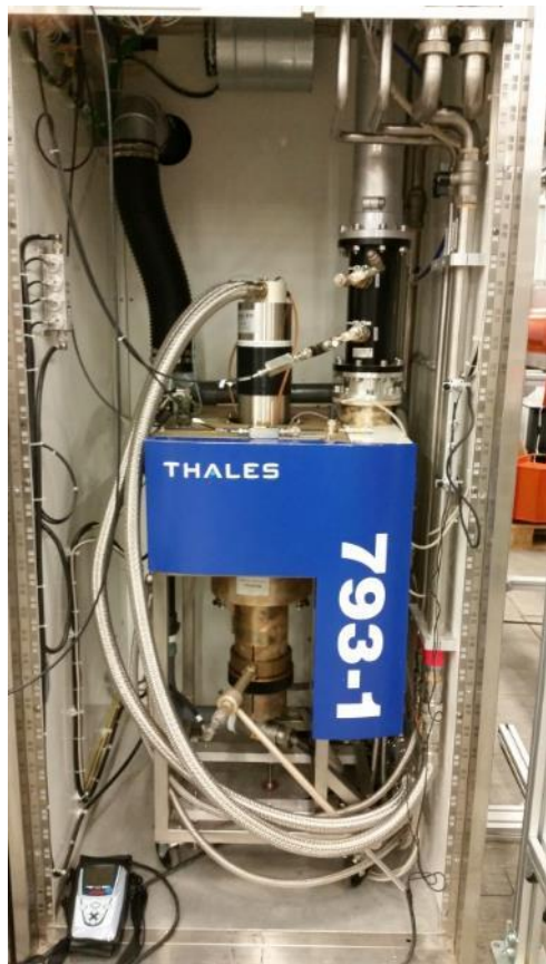
CERN SPS, TH 795 IOT, Trolley (single amplifier), and transmitter (combination of amplifiers) Two transmitters of four tubes delivering 2 x 240 kW @ 801 MHz, into operation since 2014
