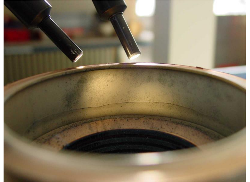
Ceramic crack due to internal metallization of the ceramic, perhaps due to over filament
