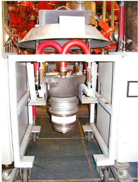
CERN SPS, RS 2004 Tetrode, Trolley (single amplifier), and transmitter (combination of amplifiers) Two transmitters of eight tubes delivering 2 \times 1 \text{ MW} @ 200 MHz, into operation since 1976
