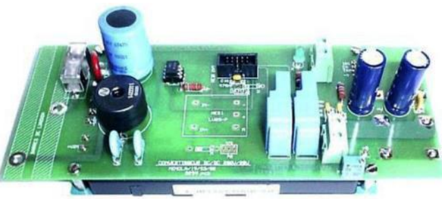
SOLEIL SYNCHROTRON elementary 600 W 300 Vdc / 30 Vdc converter board
