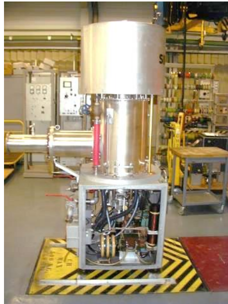
CERN SPS, RS 2004 Tetrode, Trolley (single amplifier), and transmitter (combination of amplifiers) Two transmitters of eight tubes delivering 2 \times 1 \text{ MW} @ 200 MHz, into operation since 1976
