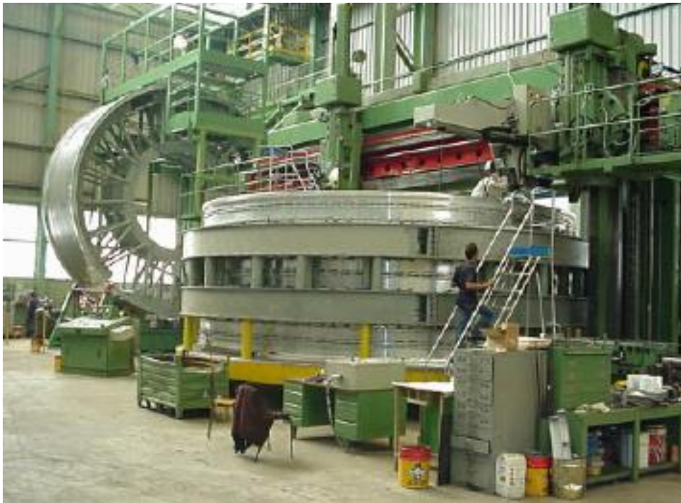
Support cylinder manufacturing, 5 units
