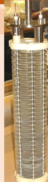
Beam-loss monitor (ionisation chamber)
