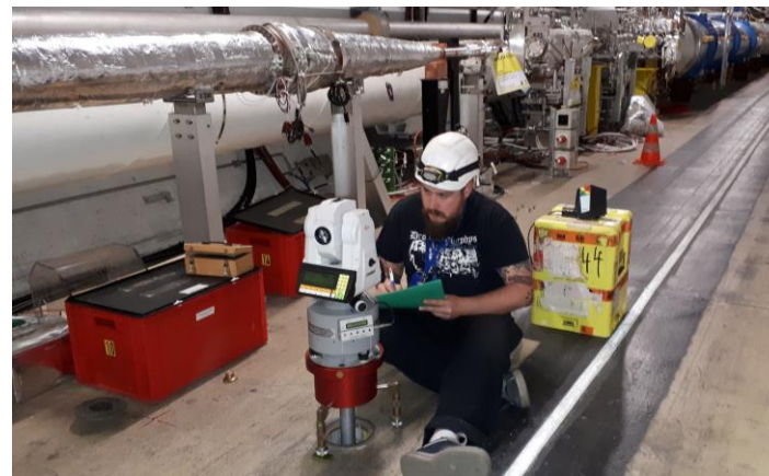
Highly accurate determination of the North direction (Azimuth)
