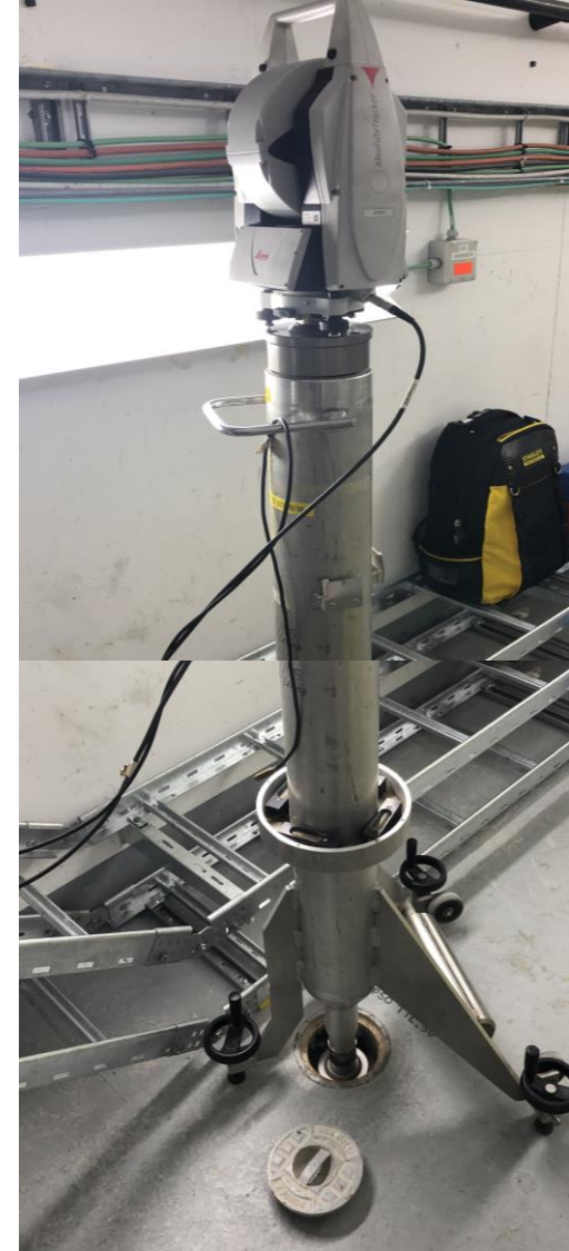
Forced centering system on a GGPSO
