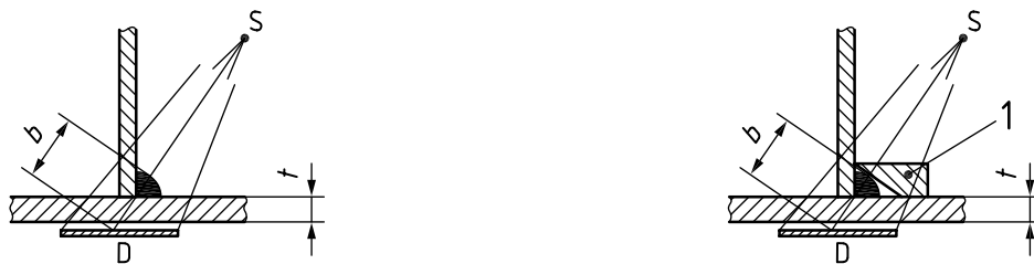
a) Arrangement for testing without compensating edge b) Arrangement for testing with compensating edge
