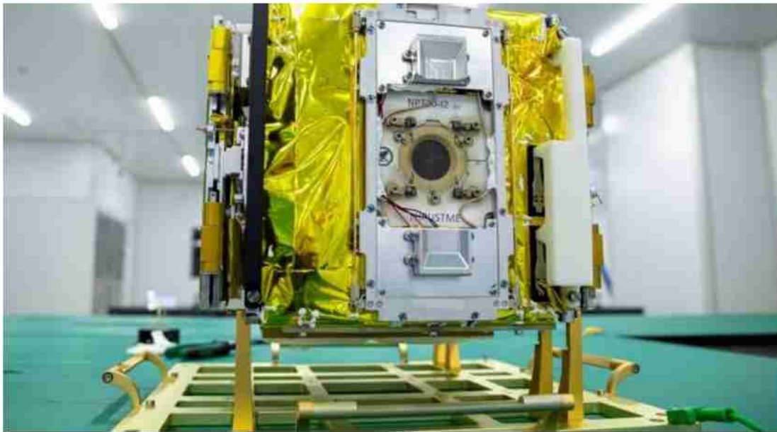
ThrustMe's NPT30-I2-1U propulsion system installed on the Spacety Beihanghongshi-1 CubeSat. Credit: Spacety
