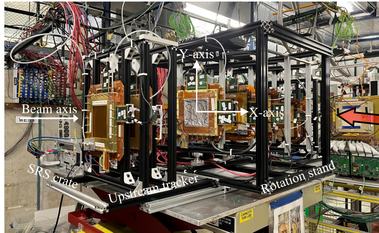
Setup II: Spatial resolution vs. angle scan setup
