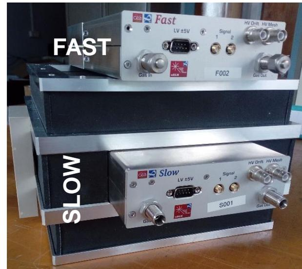
Assembly of a fast and a slow detector size  $\approx 20 \times 25 \times 25 \text{ cm}^3$  ( $\sim 14 \text{ kg}$ )
