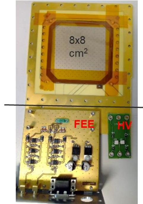
FEE board mounted on the detector
