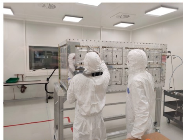
Leak test after ERAM installation
