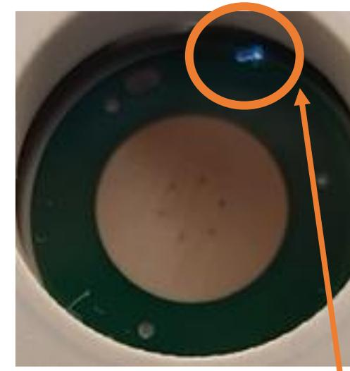
Example of discharge development in mesh cut region on a single channel prototype with a thin gap (~100 um)
