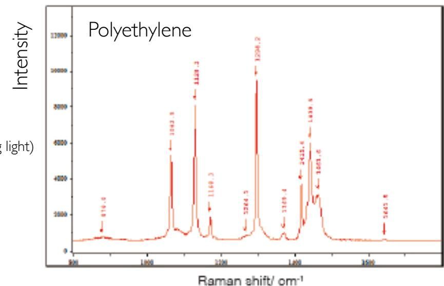
Wavenumber shift of Raman scattering light  $1/\lambda_i = \nu_i/c$
