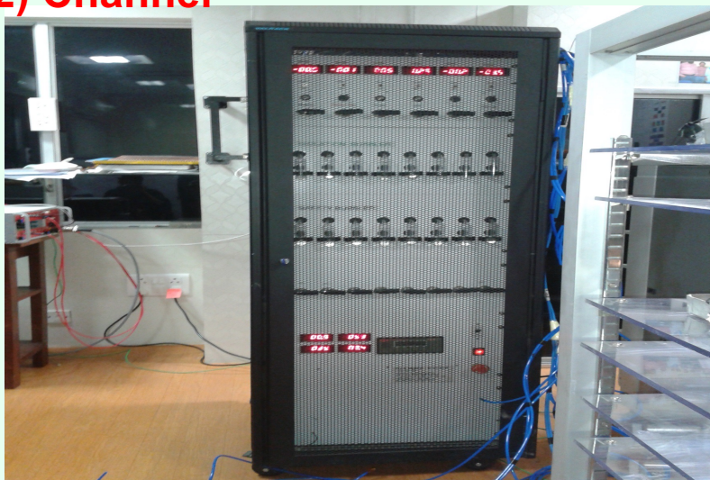
Gas Mixing Unit 6 (upgraded to 12) Channel
