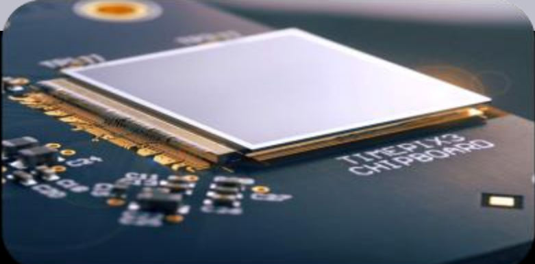
MEDIPIX Read-out chips for particle imaging
