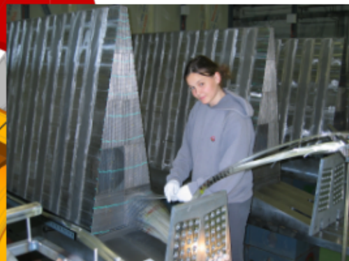
FORWARD CALORIMETER Steel + Quartz fibres ~2,000 Channels
