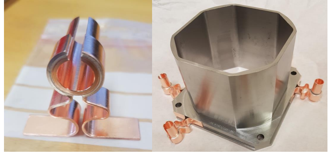
Brazing of copper/copper and copper/tungsten
