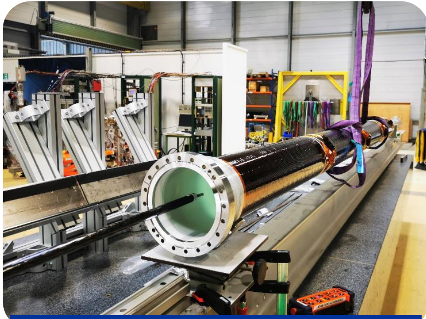
HF-CT2 Beam Pipe Endoscopic Inspection
