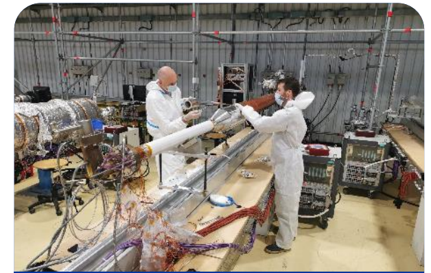
Permanent Insulation Installation
