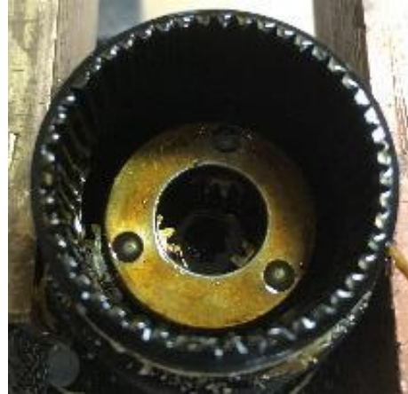
Electropneumatic motor failed at 5MGy due to brittle blades and affected grease.
