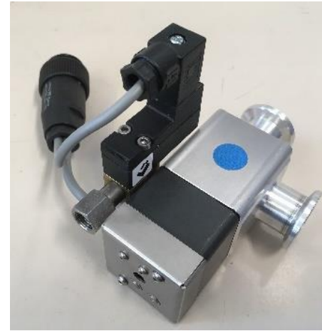
Piezo-electric distributor failed at 0.5MGy due to the piezo-electric element and leaking degraded body gaskets.
