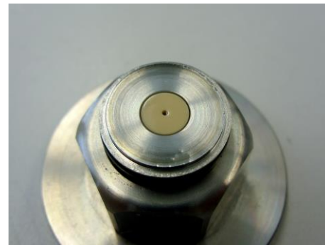
Membrane removed Discoloration of sintered ceramic
