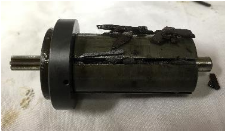
Electropneumatic motor failed at 5MGy due to brittle blades and affected grease.
