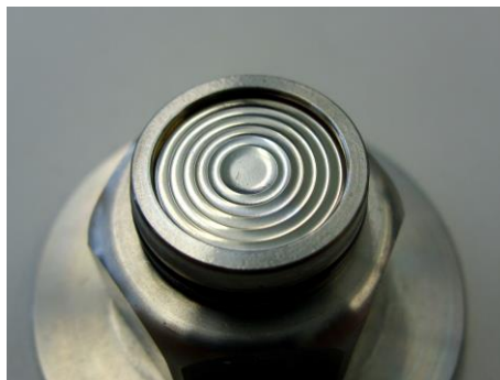
Stainless steel membrane in normal condition
