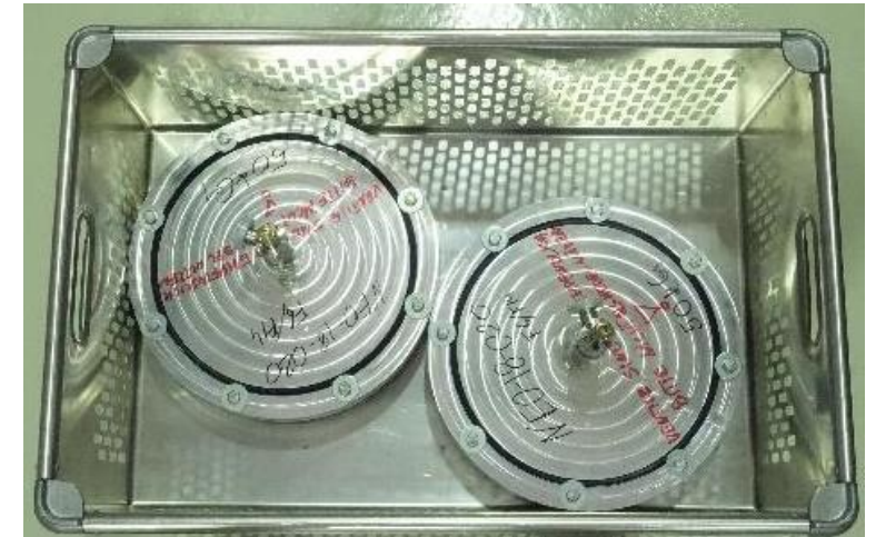
Vacuum assemblies with O-rings
