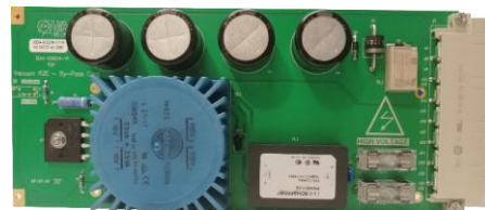
By-Pass valve local control
