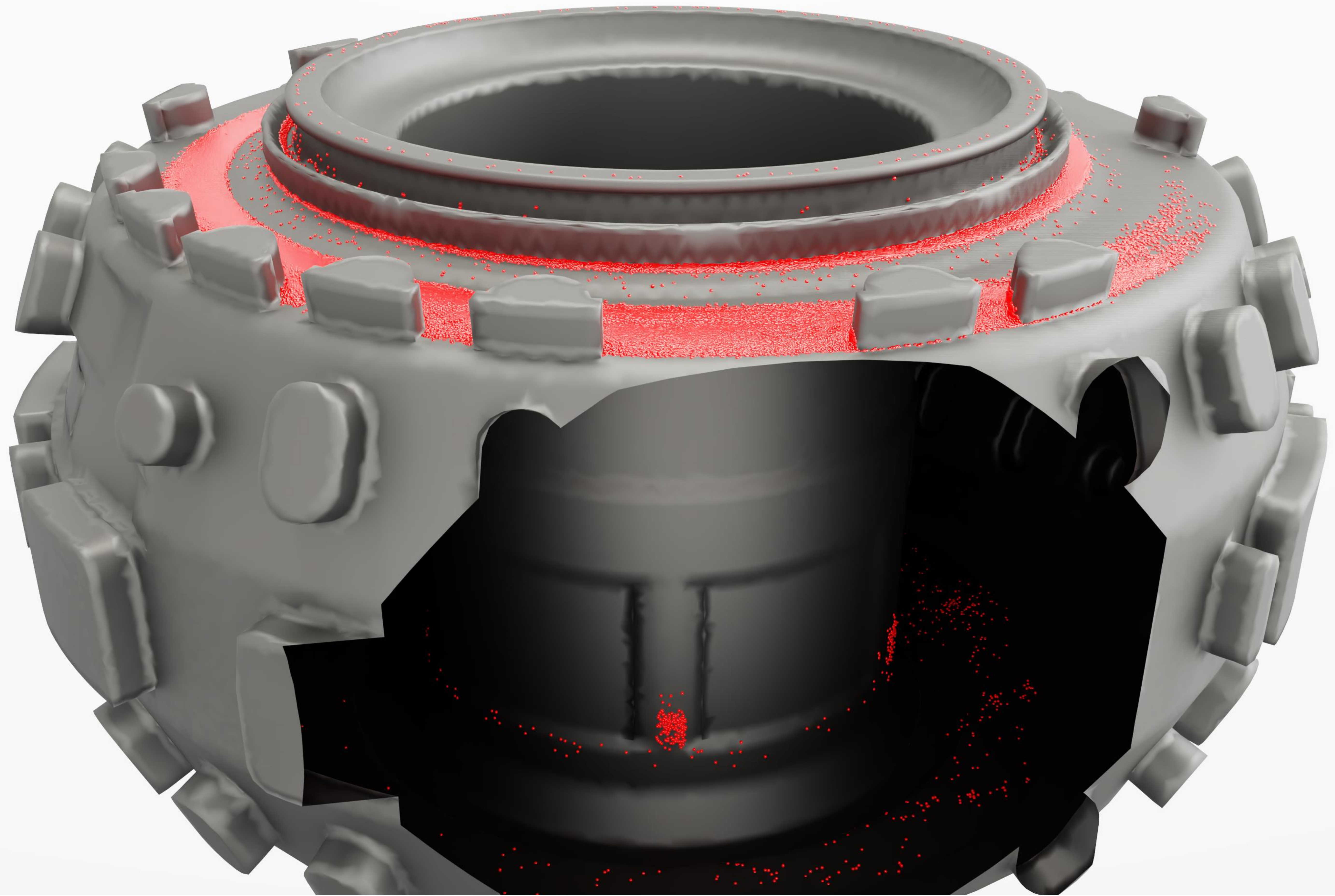
GA Ion Orbiter DIII-D Vacuum Vessel Impacts
