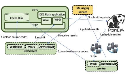
Schema of how a workflow executes a function at remote distributed resources
